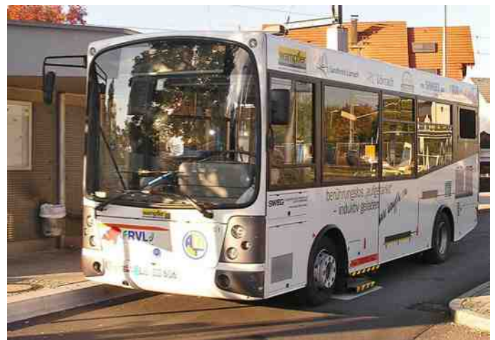
Figure 1: Contact-free recharging e-bus. All photos: City of Lörrach
